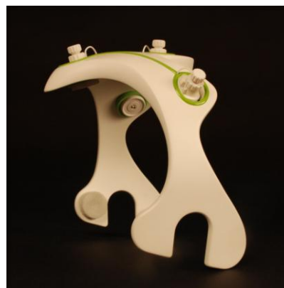
Fig. 4. Example of a BCI diadem with wires, electrodes and pre-amplifier electronics integrated (courtesy of TU Eindhoven, Department of Industrial Design). All battery-operated electronics will be integrated into the diadem and it will communicate wirelessly to an external computer or PDA that shows the stimuli and that performs the adaptation of the decoding algorithm to the subject (feature extraction and classification).
